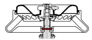
3. Let the rotor slide slowly down the centrifuge spindle.
